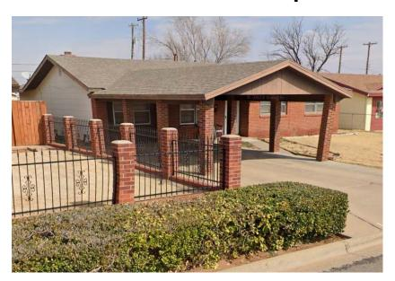
THIS CARPORT MATCHES THE ROOF PITCH, HAS THE SAME ROOFING AND SIDING MATERIALS AND IS NO CLOSER THAN 5 FEET FROM THE FRONT PROPERTY LINE. THIS MEETS THE DESIGN GUIDELINES.
